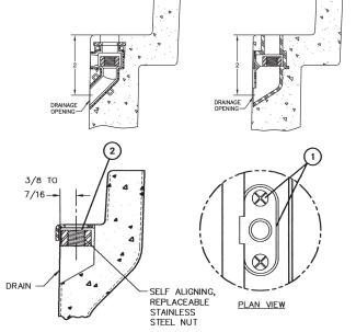
SELF ALIGNING, REPLACEABLE STAINLESS STEEL NUT
