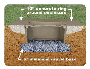
Concrete collars may be desired to give added protection to Hubbell enclosures installed by driveways, parking lots and off-roadway areas that are subject to occasional non-deliberate traffic. Concrete collars are not necessary in grassy areas or areas subject solely to pedestrian traffic.
